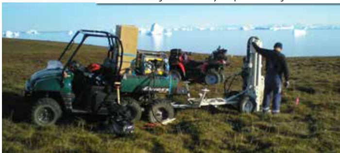
A 540MT is used for geotechnical surveys at a potential mining site in Greenland.
