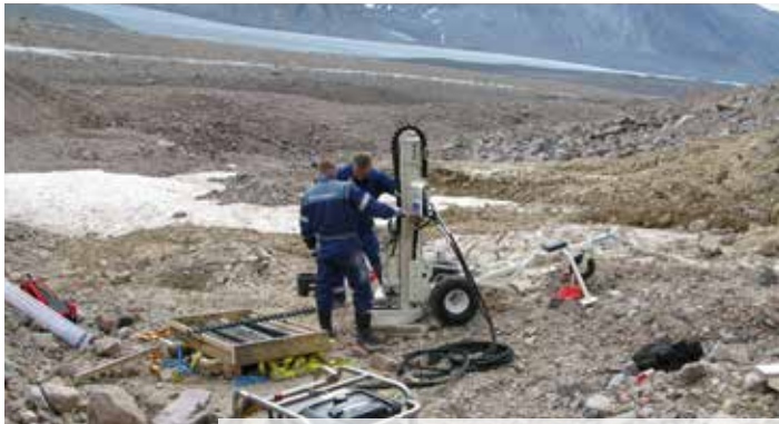
A 540MT is used for geotechnical surveys at a potential mining site in Greenland.
