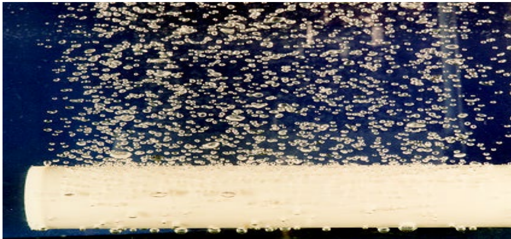
Figure 1: Bubble pattern as air is passed through a SCHUMASOIL well screen
