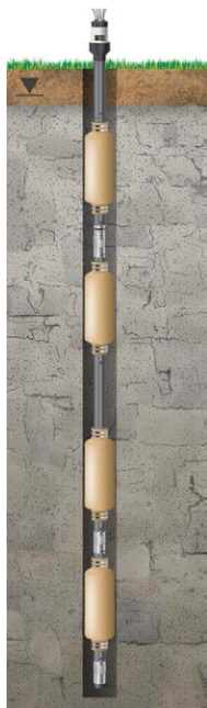
Waterloo System in Bedrock Using Permanent Packers
