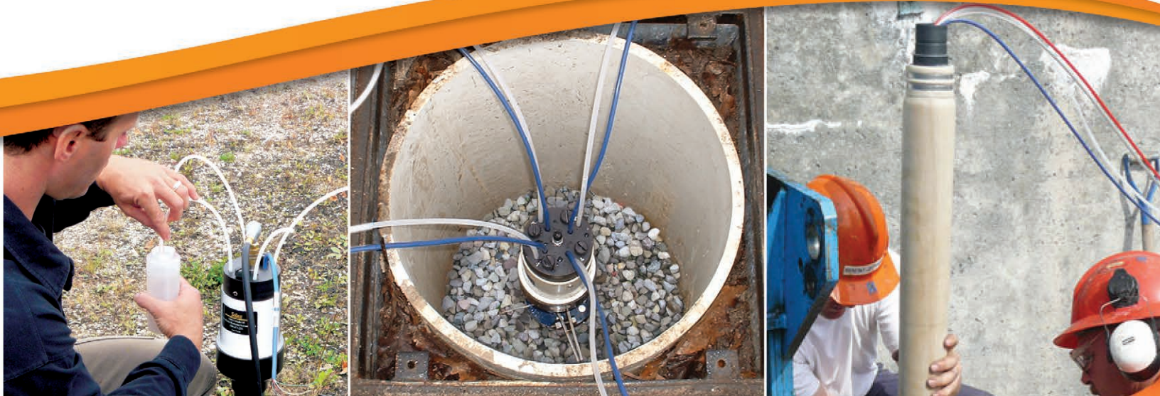
Waterloo System in Bedrock Using Permanent Packers
